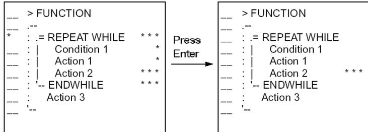
If a pair of \*\*s is used, these must be defined at the same construct level. Each construct at the same level as the \*\* has its associated active/deactive flag toggled. This can lead to some constructs being deactivated and some being reactivated. Constructs nested within these constructs are not updated but still inherit the deactivation of their parent constructs.
